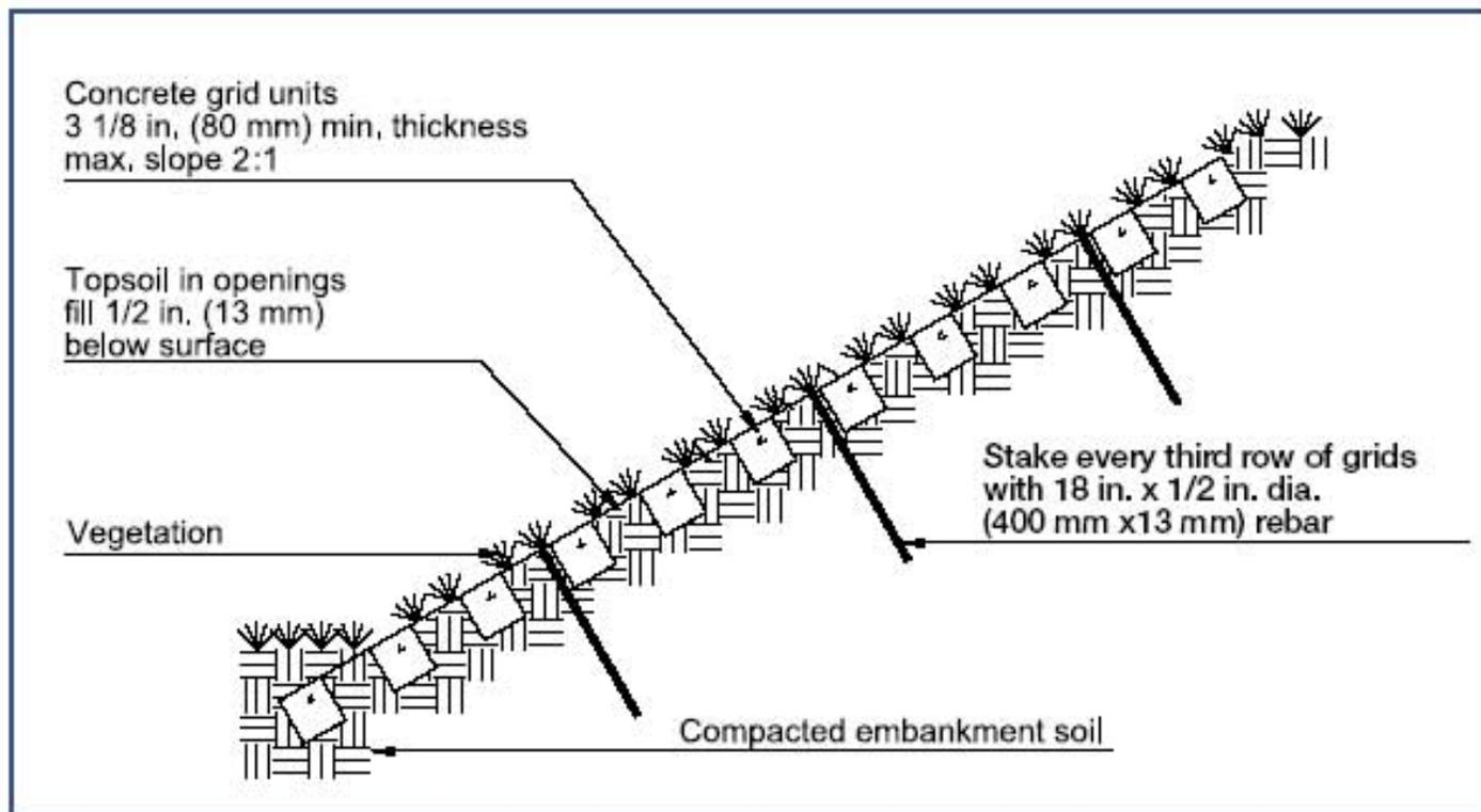
Figure 19. Embankment stabilization with concrete grids
