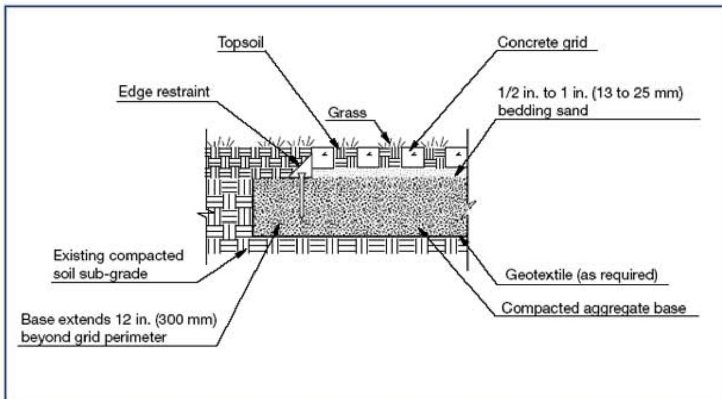
Figure 17. Typical concrete grid pavement over dense-graded base
