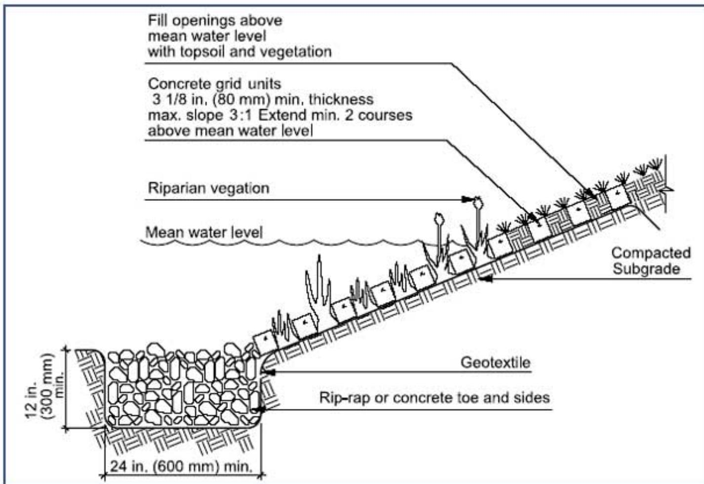
Figure 21. Lake side stabilization with concrete grids
